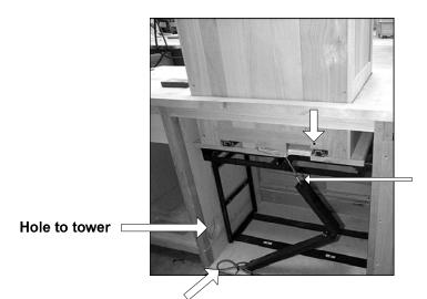
Keyboard, mouse and monitor power supply cords must be threaded through this black plastic raceway. Then trough the hole to the tower.
